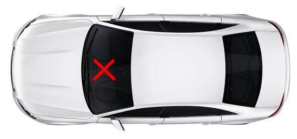
If the measurements are taken in a vehicle other than a car, when installing the device, consider that for consistent GPS/GLONASS reception, the backside of the device should be directed upwards. For improving the quality of reception, avoid placing other electronic devices (radar detection device, tablet PC, smartphone) close to the area where the Race Meter is attached.
