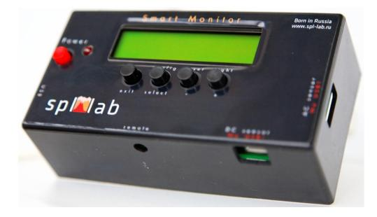
Smart Monitor from Spl-Lab will protect your car audio components from damage, will help in tuning sound in the car, as well as will measure power of your sound system and acoustics characteristics. The Smart Monitor replaces amp clamp, True RMS digital voltmeter and oscilloscope. And, in addition to this, provides protecting functions.
